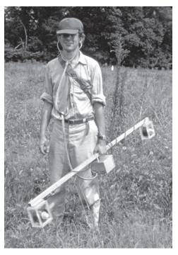
Vin and his differential proton magnetometer exploring the Haynes Bluff site, 1974 (LMS photo).
